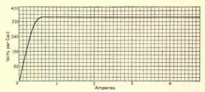
Frg. 174.—Graph showing how the electrolytic protector permits current to flow readily at pressures above 330 volts per cell.
